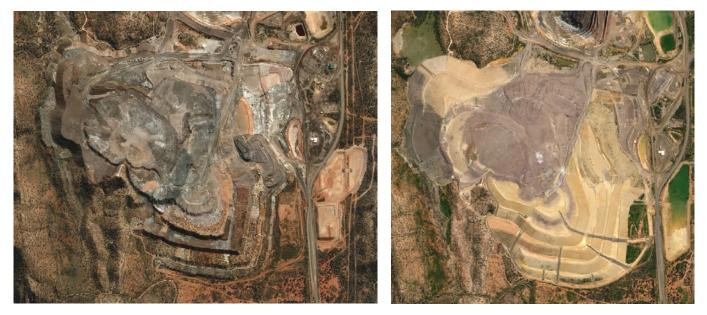
Satellite imagery of Handlebar Hill Mine in Queensland, displaying mine rehabilitation progress between 2016 (left) and 2023 (right). Supplied by Geoimage Pty Ltd. © Airbus DS (2016) / © Airbus DS (2023).
