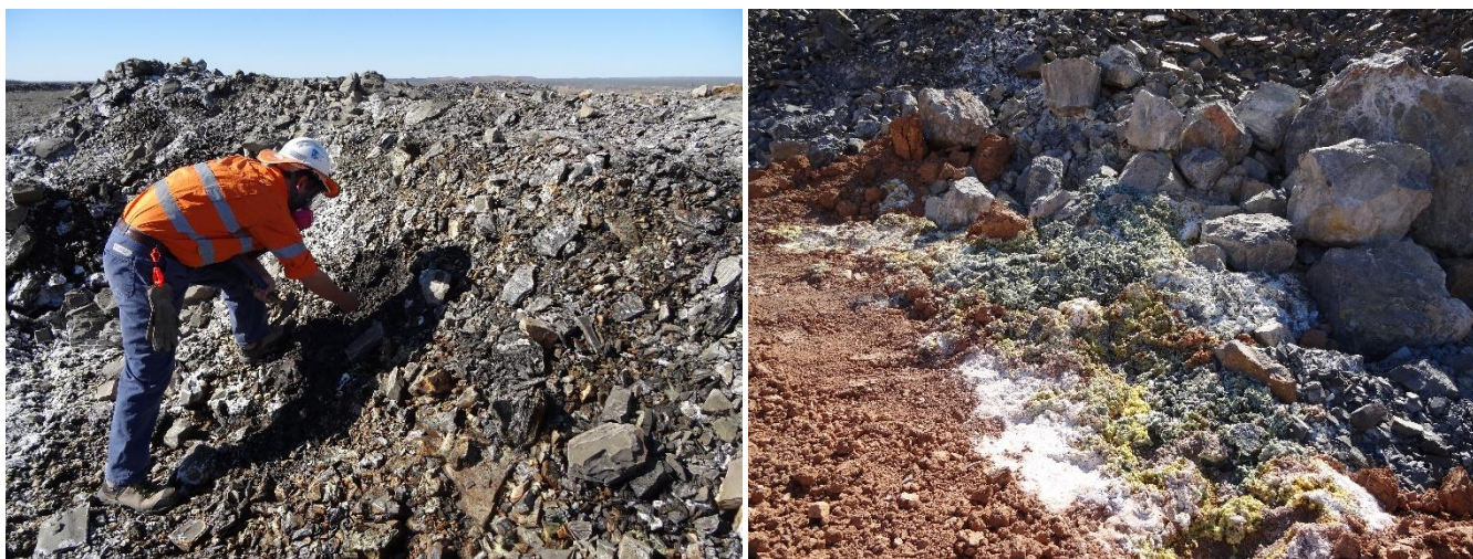
Figure 35: Oxidation of sulfidic waste rock exposed on the North Overburden Emplacement Facility
