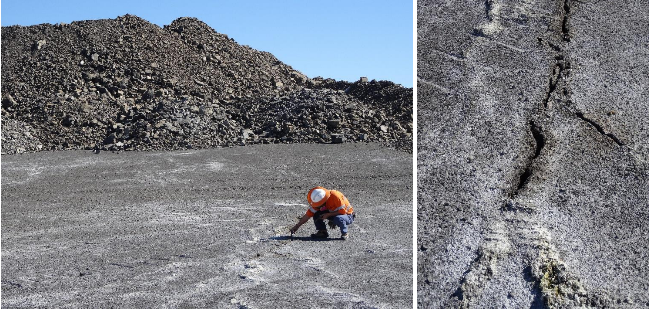
Figure 36: Breakthrough of a compacted rock layer due to spontaneous combustion of thinly-covered sulfidic waste rock
